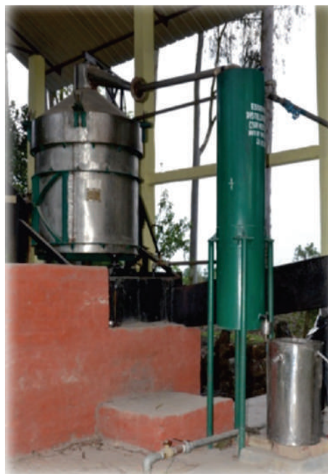
Essential oil distillation unit (300 L/Day) at CSIR-NEIST experimental farm
